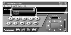
Select the camera for setting from the pull-down menu for the camera.
